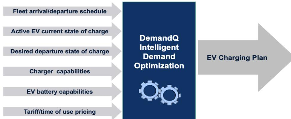
DemandQ manages EV generated peak demand at the point of charge, maintains on-time operational objectives of fleet management, and ensures fulfillment of the target charge state of each EV in the fleet.
